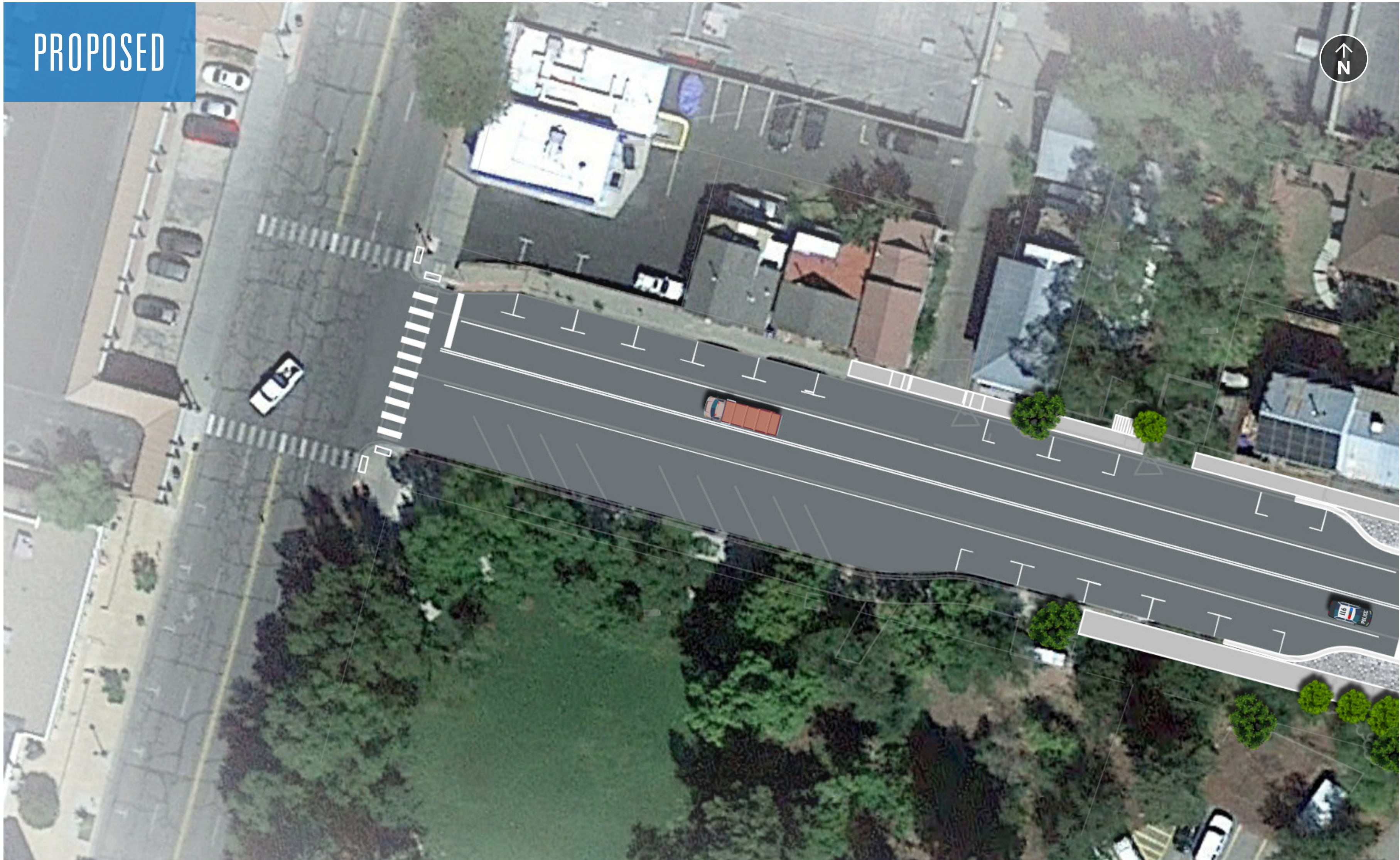
At the corner of 13th Street and Main Street, the proposed design features new detectable warning plates for the crosswalks. To the east of the intersection, both the north and south sides of 13th Street have proposed sidewalk improvements. Roadway striping and parking will match the existing configuration.
