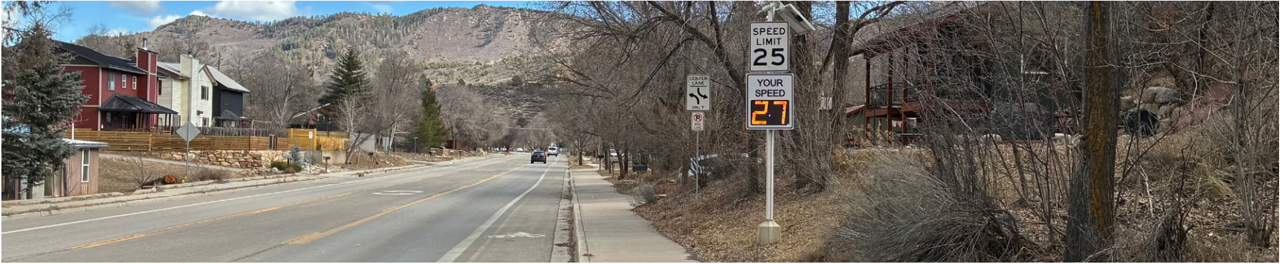
Photo 31. Speed Feedback Radar Sign
